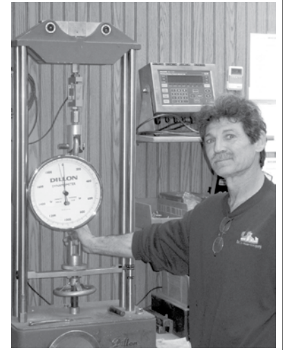
Steve Kohner with a dynamometer, which measures mechanical force.
